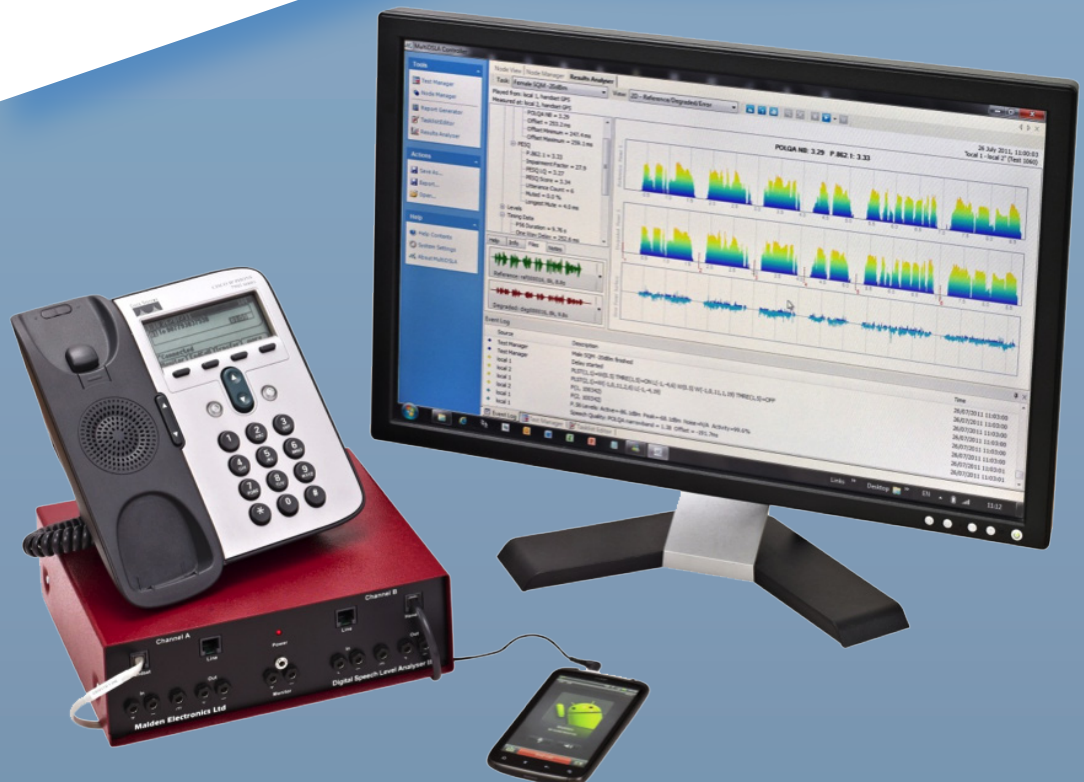
Figure 1: Typical configuration with analogue test interfaces
